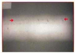
Radiographic Test is used to inspect almost any material for surface and subsurface defects. X-rays can also be used to locate and measure internal defects, confirm the location of hidden parts in an assembly and to measure thickness of materials
